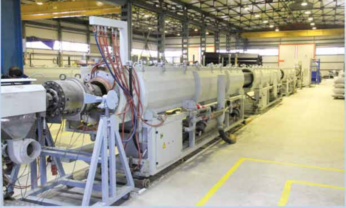
POLYETHYLENE PIPE MANUFACTURING LINE
